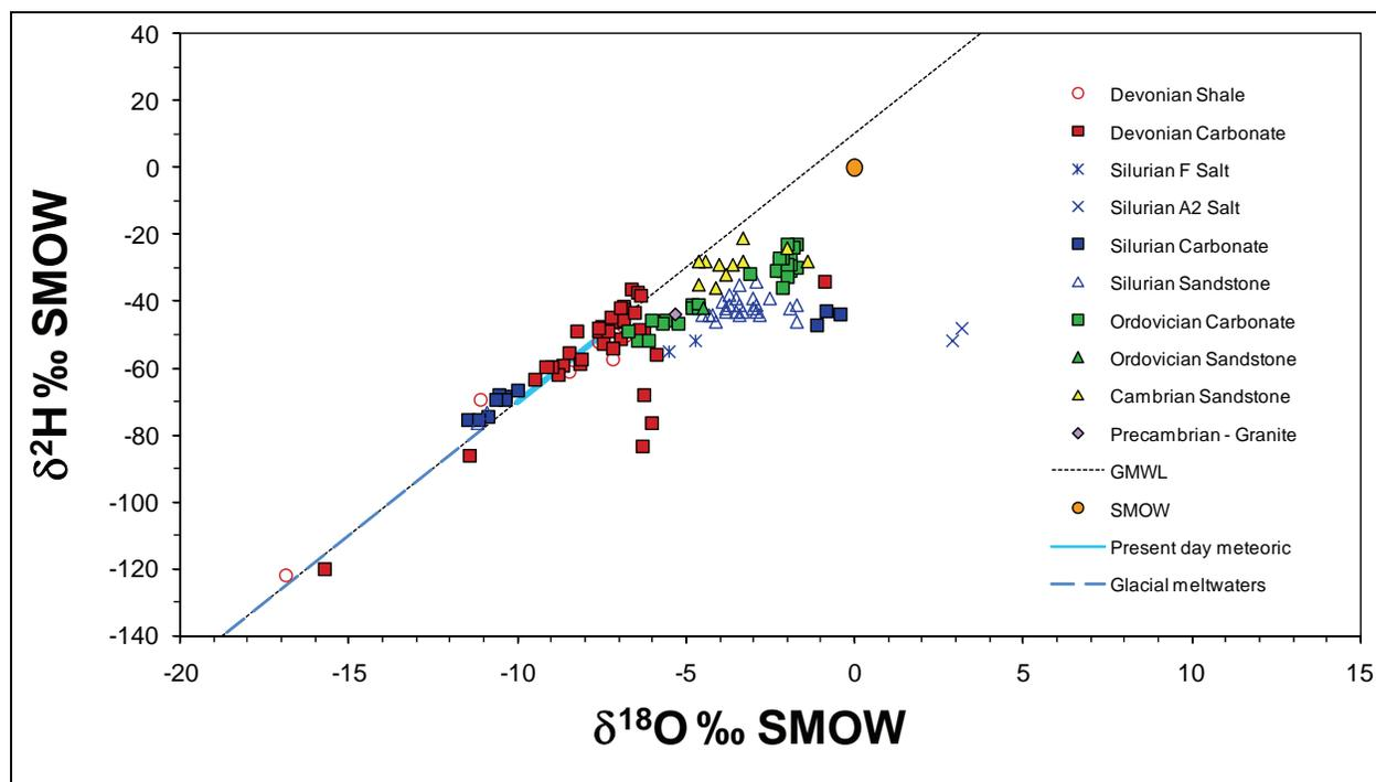
**Figure 5.8 Hydrogen versus oxygen isotopic signatures for all fluids within the UW hydrogeochemical database.**
