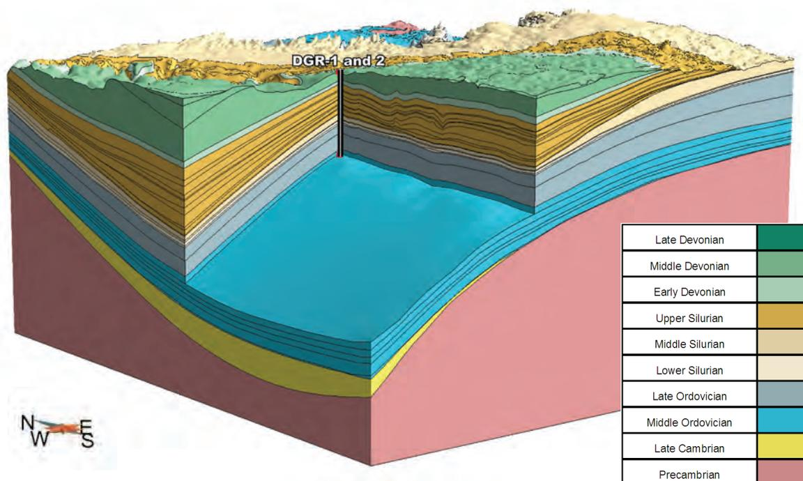
**Figure 3.12 3D Regional Geological Framework and the Location of the DGR beneath the Bruce Site (approx. 40X vertical exaggeration).**
