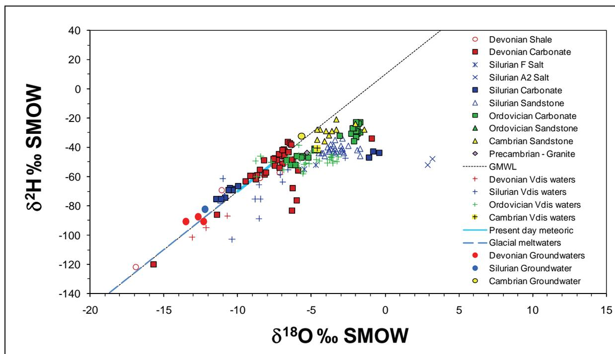
**Figure 5.11 Stable O and H isotopic data from regional groundwater sampling in southwestern Ontario (UW database) and from site characterization at the Bruce site (Clark et al. 2008). “Vdis waters” are waters from the rock matrix obtained by vacuum distillation.**
