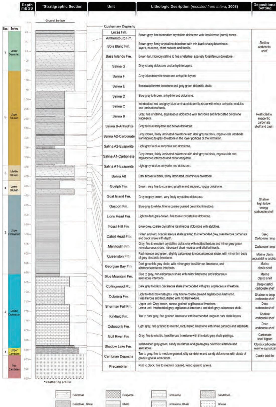
Figure 3.14 Phase I Deep Drilling Program: DGR-series boreholes – Stratigraphy
