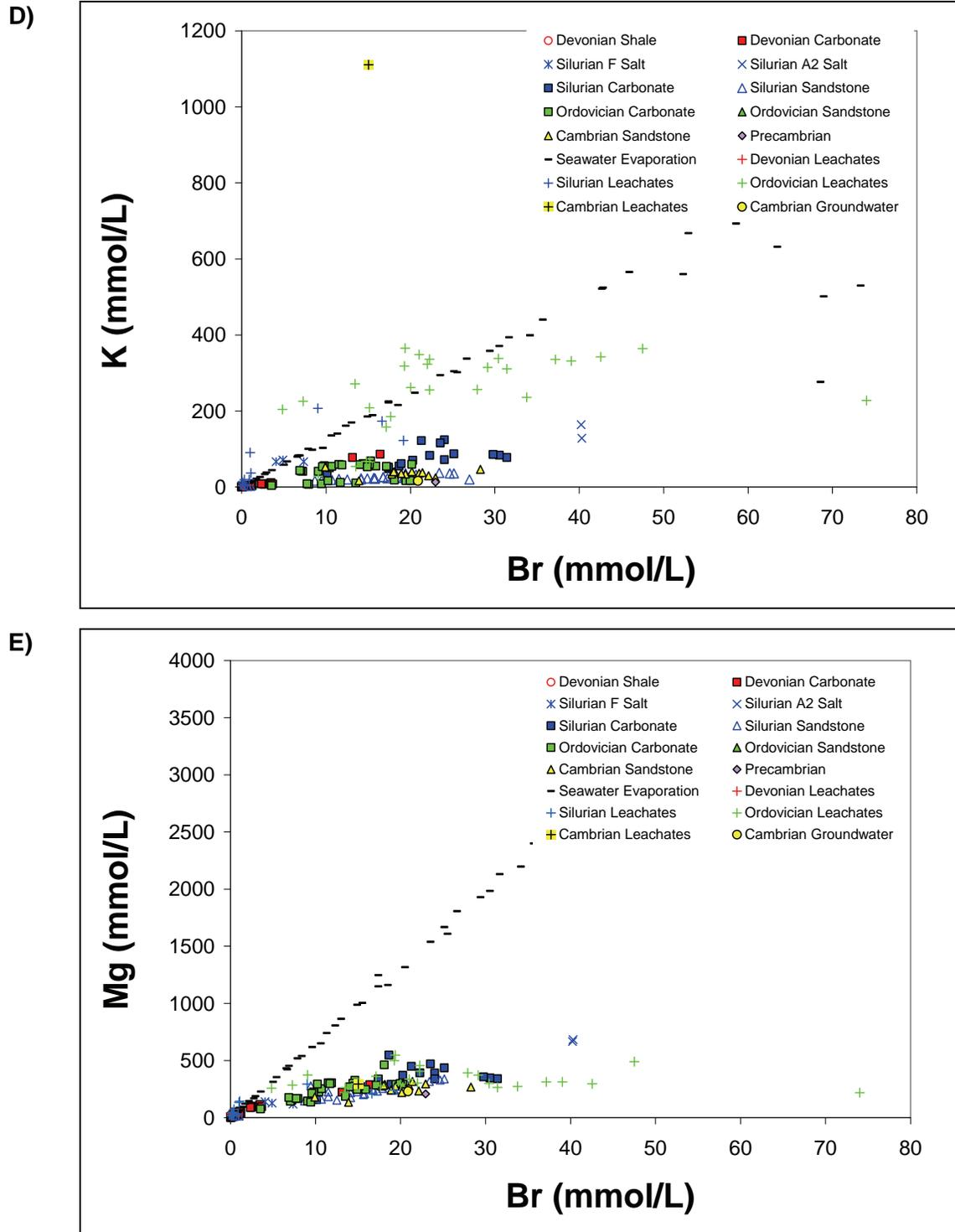
Figure 5.10 Comparison of major ion concentrations versus Br for leachate solutions from drill cores DGR1 and DGR2, with groundwater data from the UW database.
