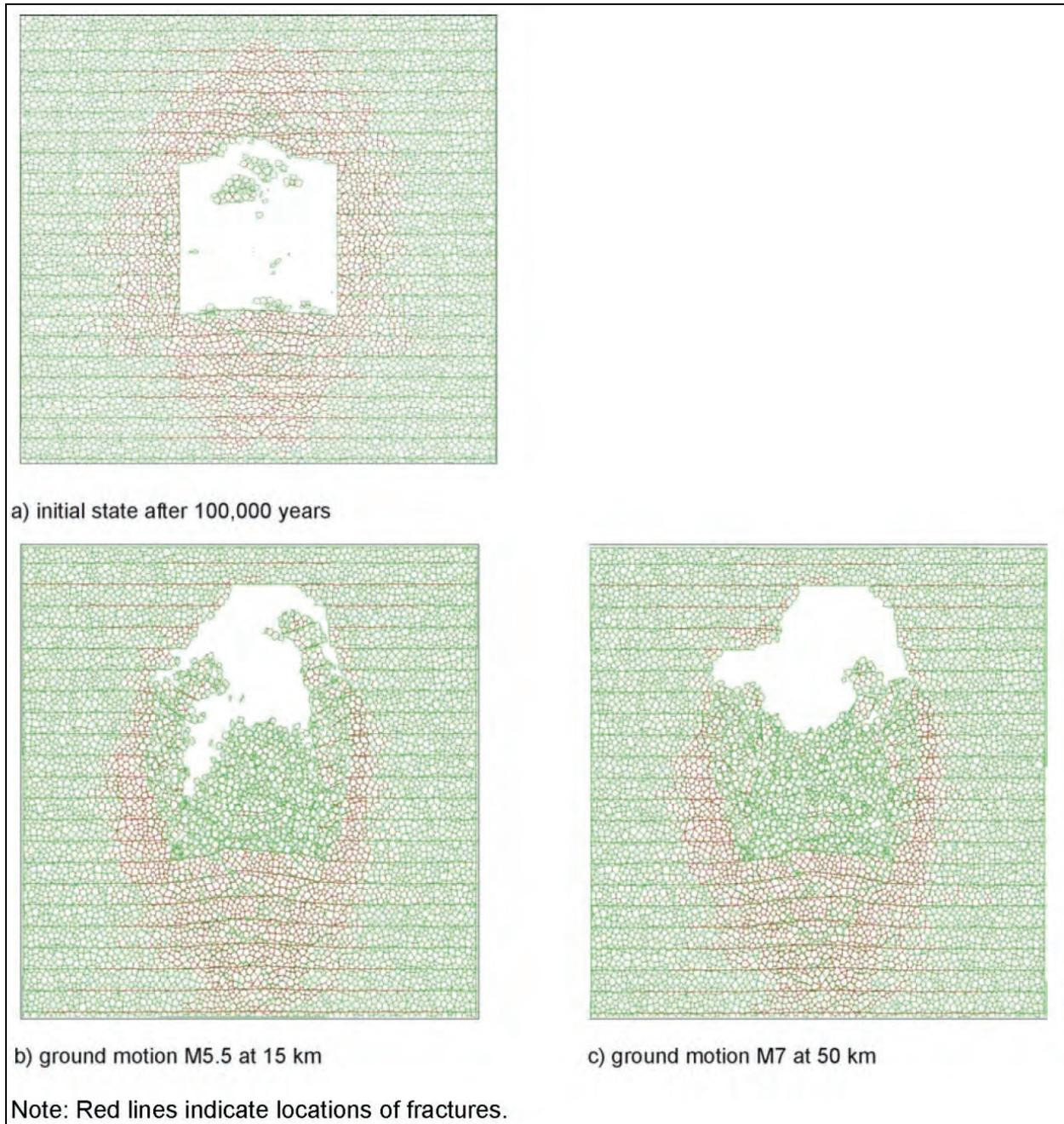
**Figure 4.13 Effects of Seismic Ground Motions after 100,000 Years of Time-Dependent Strength Degradation (Itasca, 2008)**
