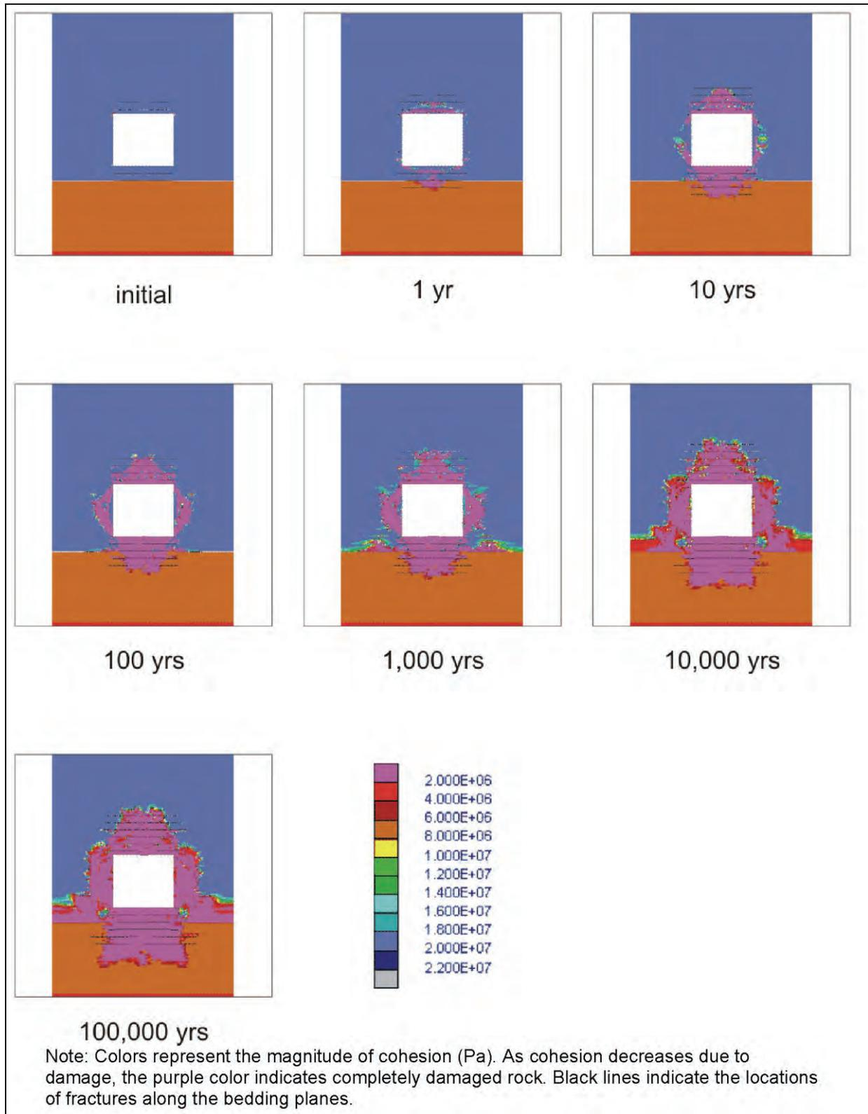
**Figure 4.12 Time-Dependent Strength Degradation Plus 13 MPa Gas Pressure Build-up Damage around the Cavern Outline (Itasca, 2008)**
