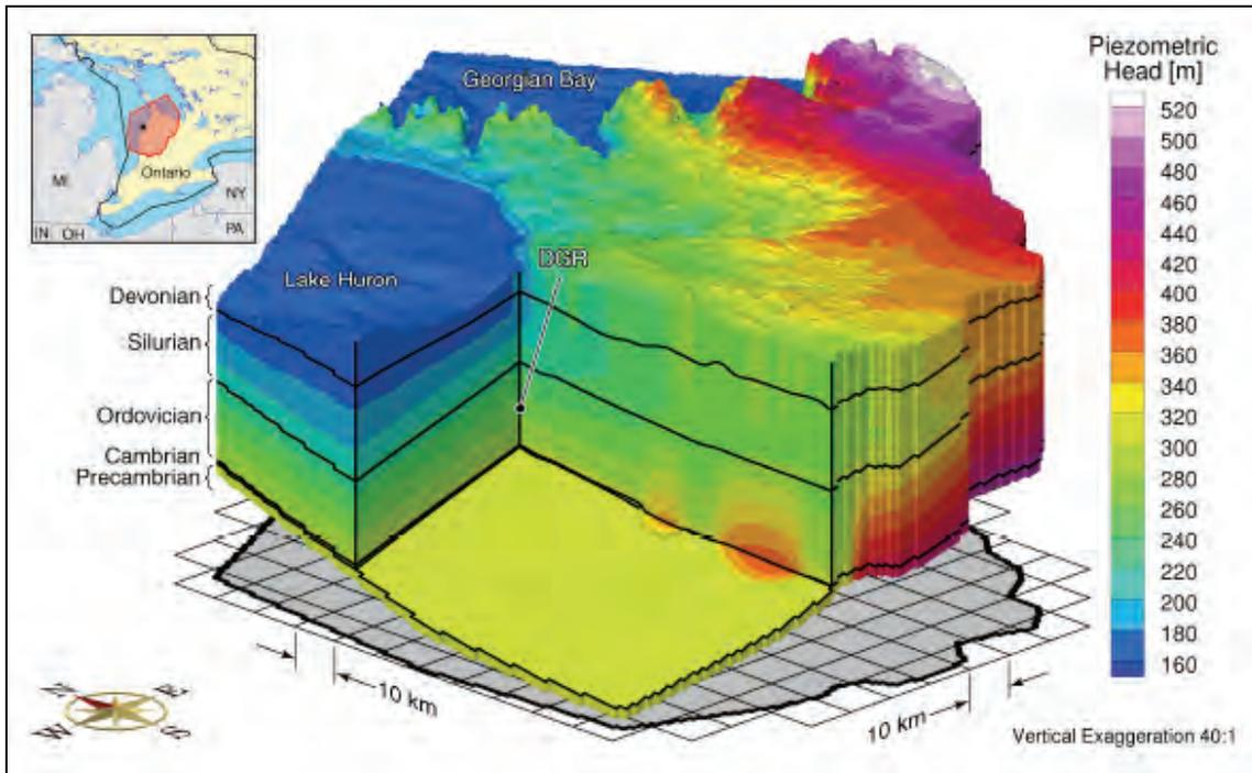
Figure 6.2 Base case equivalent freshwater head (m) distribution.
