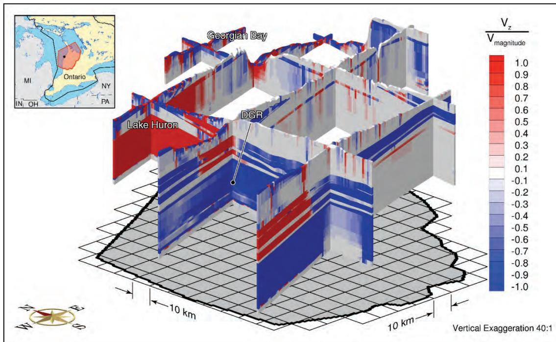
**Figure 6.6 Fence Diagram of Base Case Ratio of Vertical Velocity to Velocity Magnitude**
