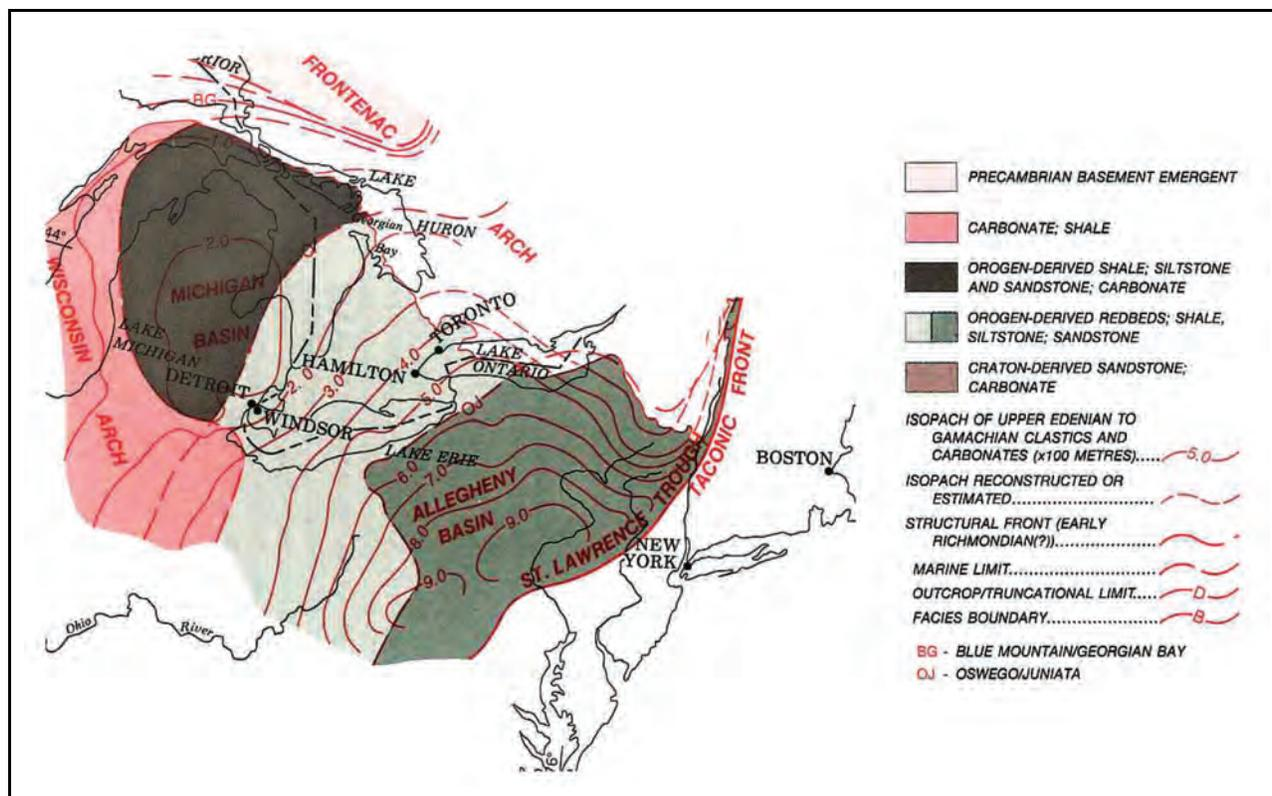
**Figure 3.9 Upper Ordovician Depositional Sequence and Isopach Thickness (Sanford, 1993)**
