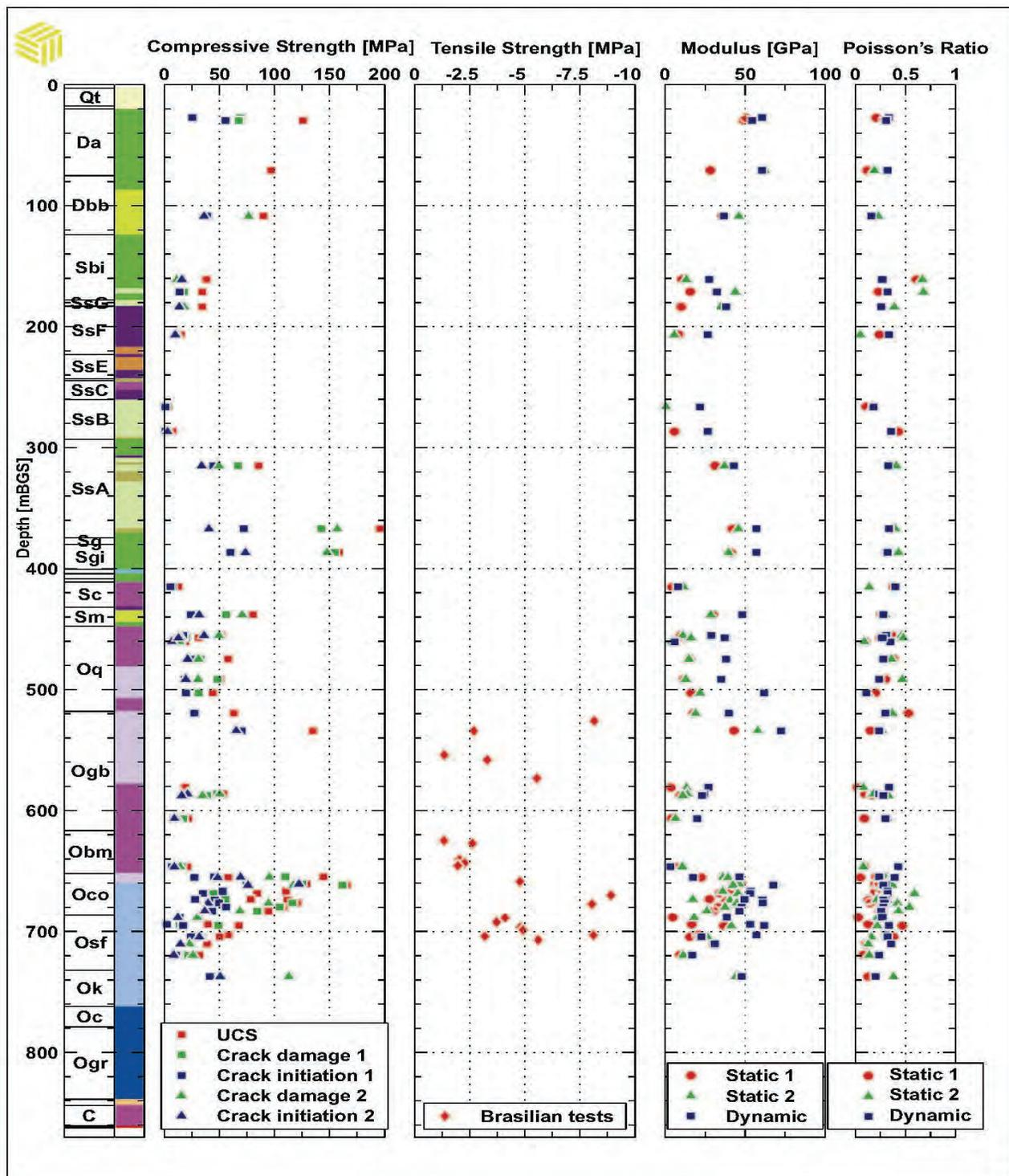
Figure 4.5 Strength and Elastic Properties measured on DGR-1 and DGR-2 Cores (Intera, 2008b)
