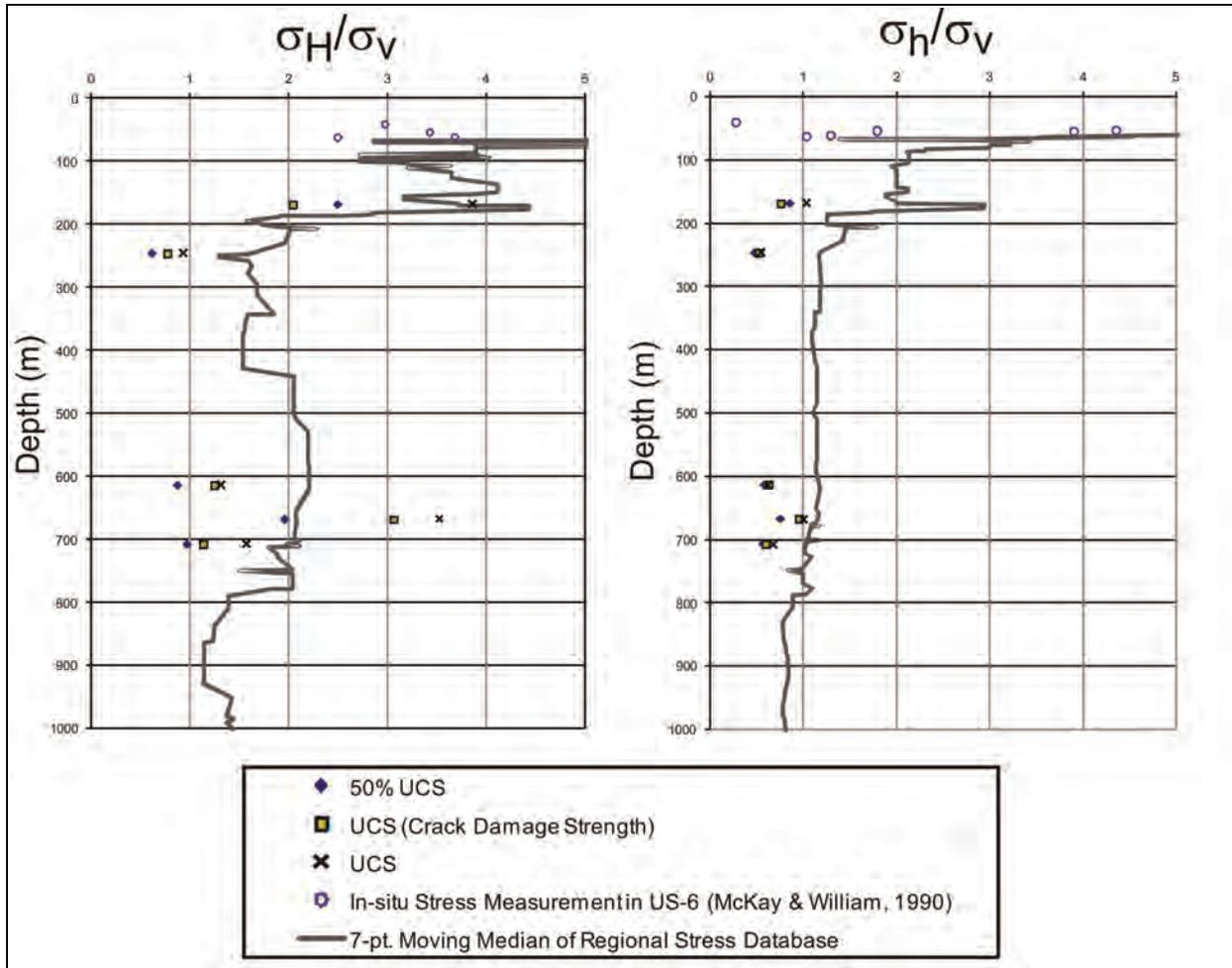
**Figure 4.9 Comparison of stress constraints and overcoring stress measurements at the Bruce Site with regional data. Grey solid line is the moving median in-situ stress ratio derived from regional data at 20 sites (Gartner Lee Limited, 2008b).**
