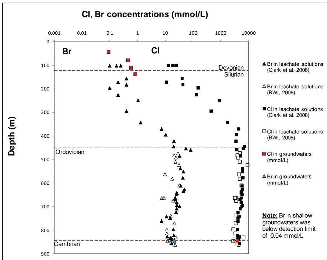
**Figure 5.9 Profiles of Cl and Br concentrations in groundwater and in waters extracted from the rock matrix (leachate solutions).**
