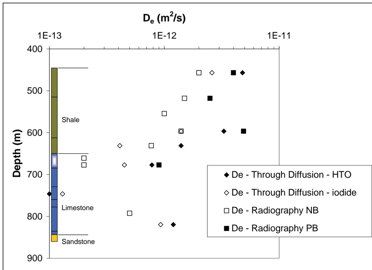
**Figure 5.13 Results of laboratory-scale effective diffusion coefficient measurements conducted by Al et al. (2008). All radiography measurements are conducted with iodide tracer (NB = normal to bedding; PB = parallel to bedding).**
