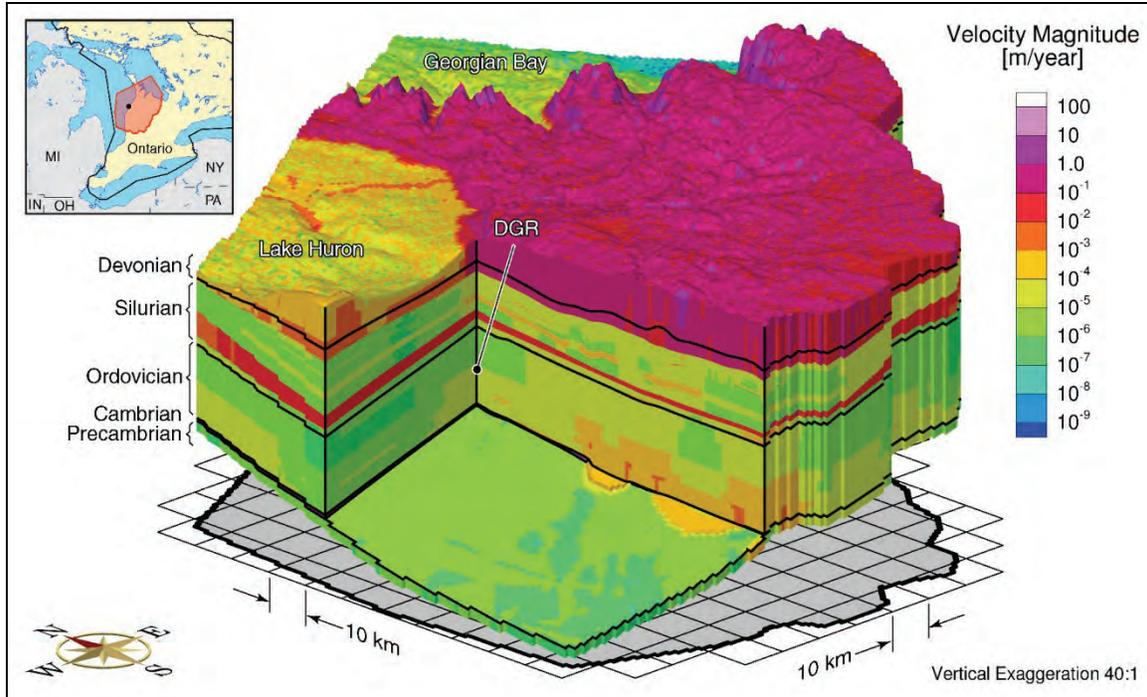
Figure 6.5 Base Case Pore Water Velocity Magnitude Distribution
