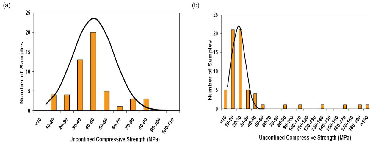
**Figure 4.3 Unconfined Compressive Strength of; (a) Queenston and (b) Georgian Bay Shales (Gartner Lee Limited, 2008b)**
