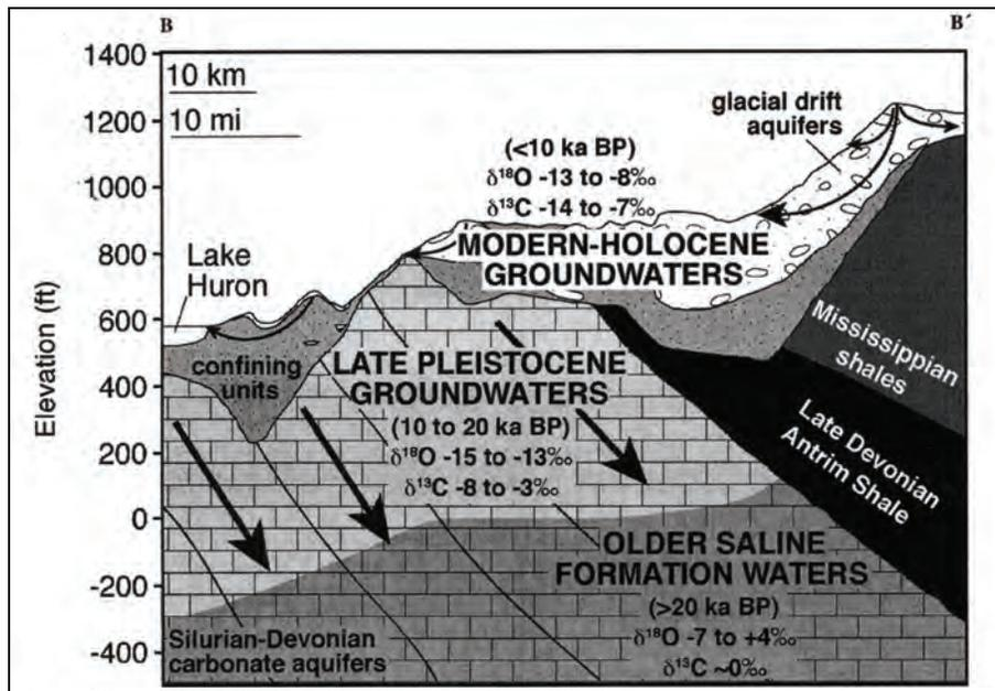
**Figure 5.7** Conceptual model developed by McIntosh and Walter (2006) showing ancient brine at depth, cold-climate water recharged during the Pleistocene at mid depths, and modern meteoric water near the surface.
